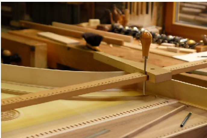
Figure 14. Marking bridge pin positions.
