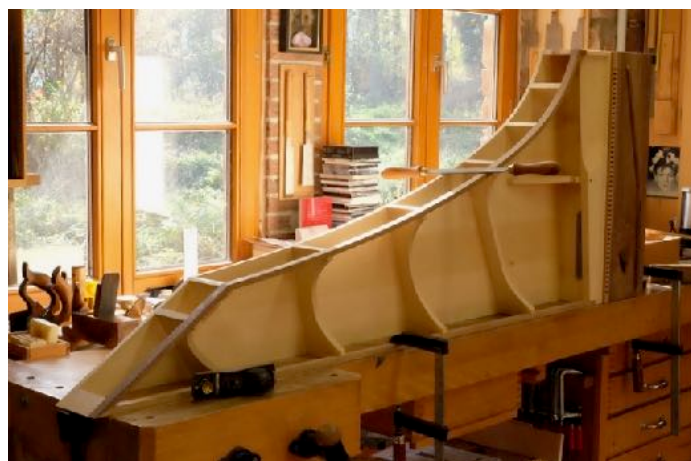
Figure 11. Neapolitan model with spruce framing and acute tail; note the double-handled rasp for fairing the bentside frame.
