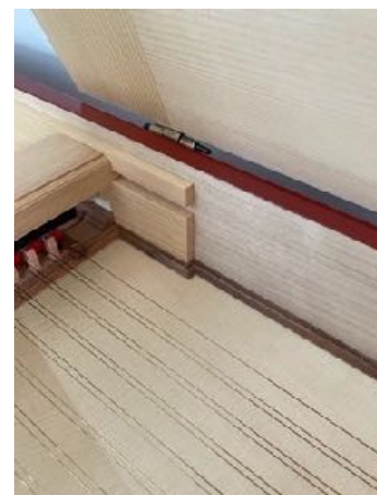
Figure 20. Thick veneer doubles as wrestplank hold-down and jack-rail support block.
