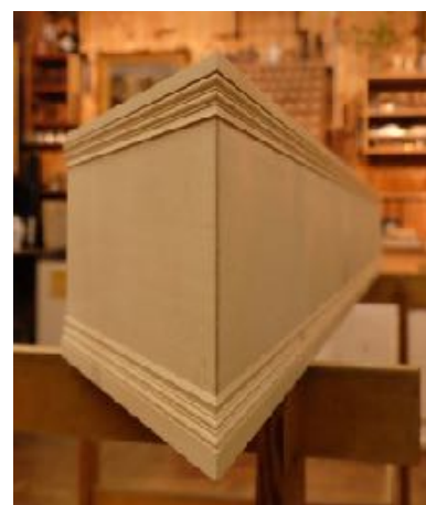
Figure 12. Butted tail joint with mitred mouldings.
