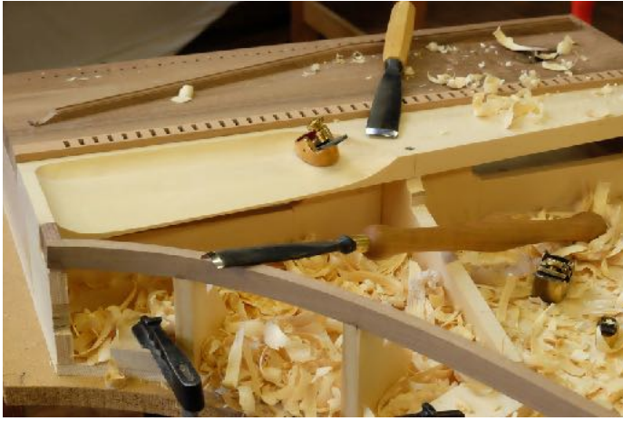
Figure 13. Secondary ‘wrestplank’ hollowed out to free up soundboard.
