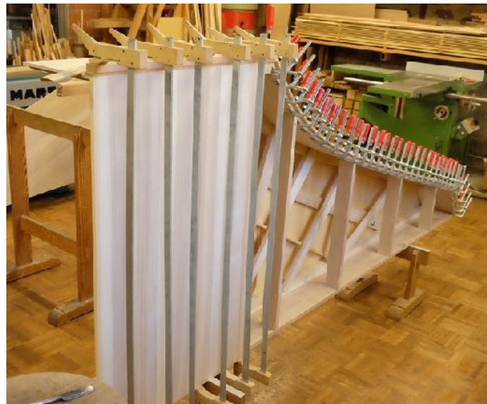
Figure 7. Front part of bottom panel installed, but soundboard is still accessible from below.
