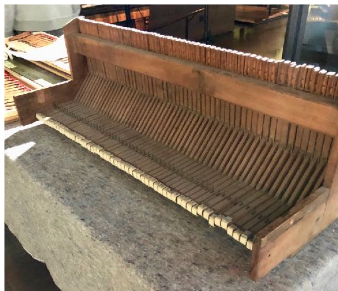
Figure 3. The bell-crank chassis of the Brussels instrument with key-dip limiter removed.
