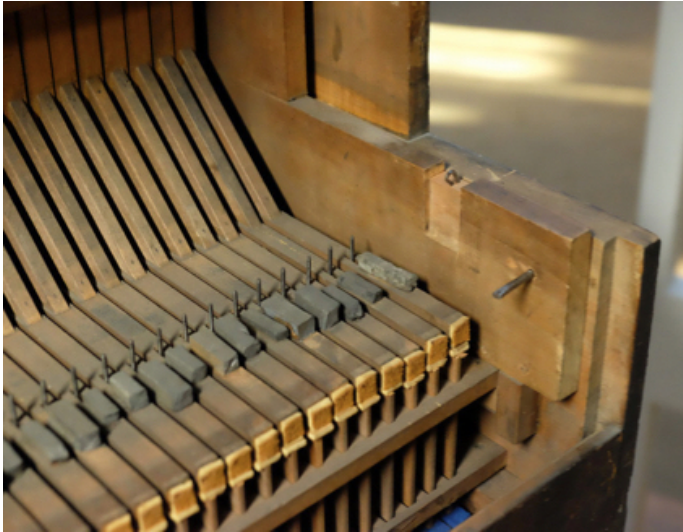
Figure 5. Lead weights on the bell-cranks of Berlin [photo: courtesy of M. Griewisch].
