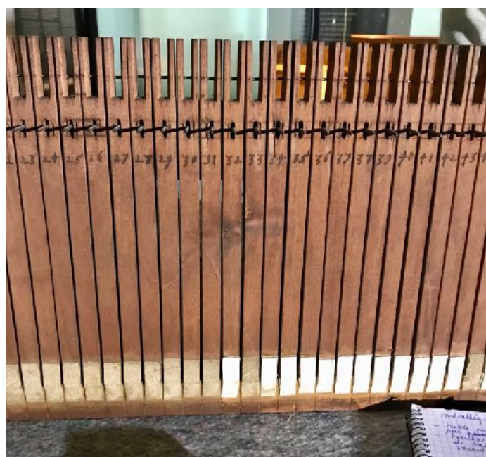
Figure 8. Delin's action: the shake or knot running from rocker arms 31 to 34 shows they were cut from a single plank.
