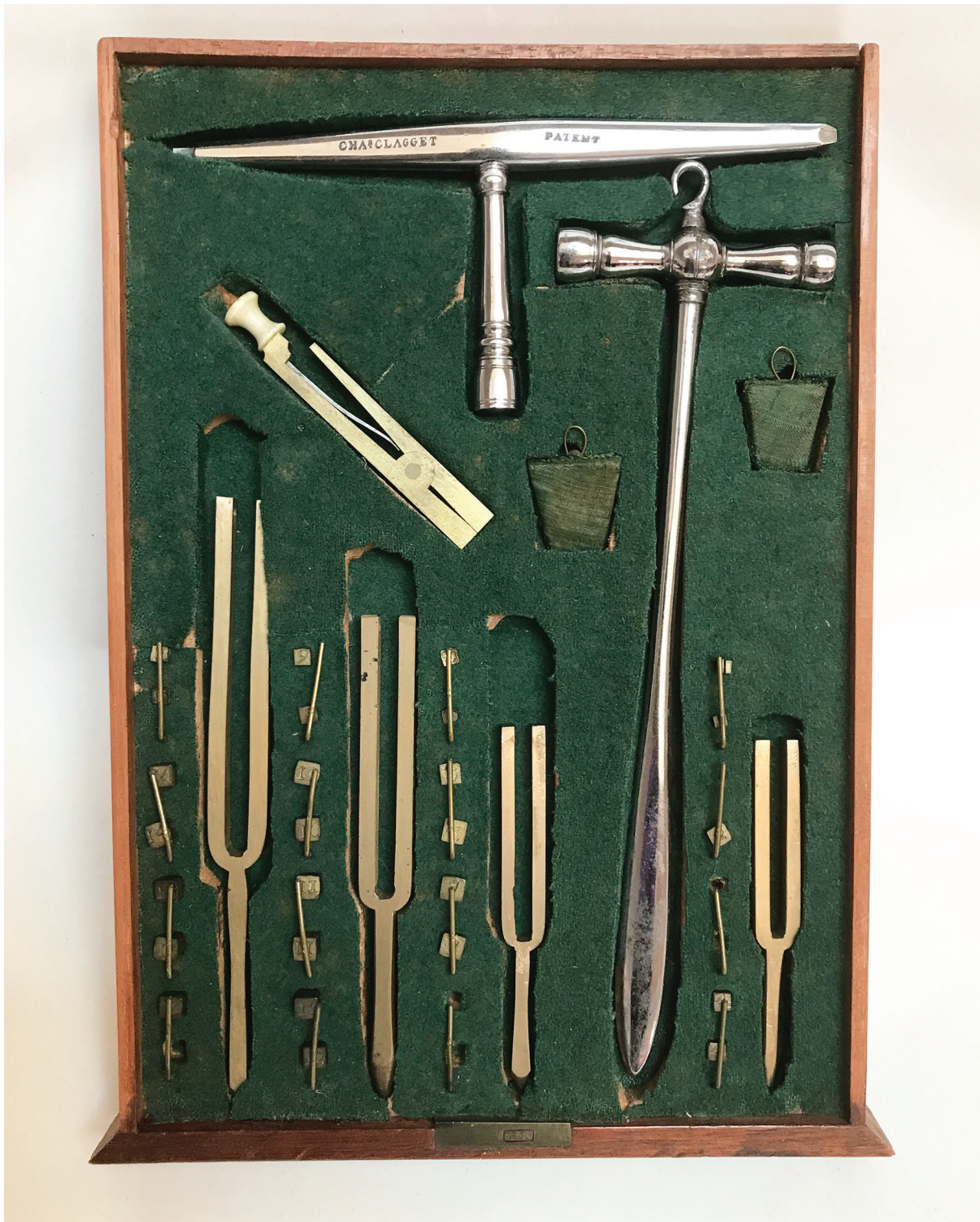
Figure 4. Tuning set of forks and weights plus tuning hammers by Charles Clagget, The University of Edinburgh (MIMEd 6407), © The University of Edinburgh.
