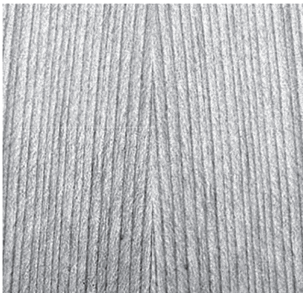
Figure 5. Appearance of the central joint of spruce in the case of a tapered reduction of the soundboard.
