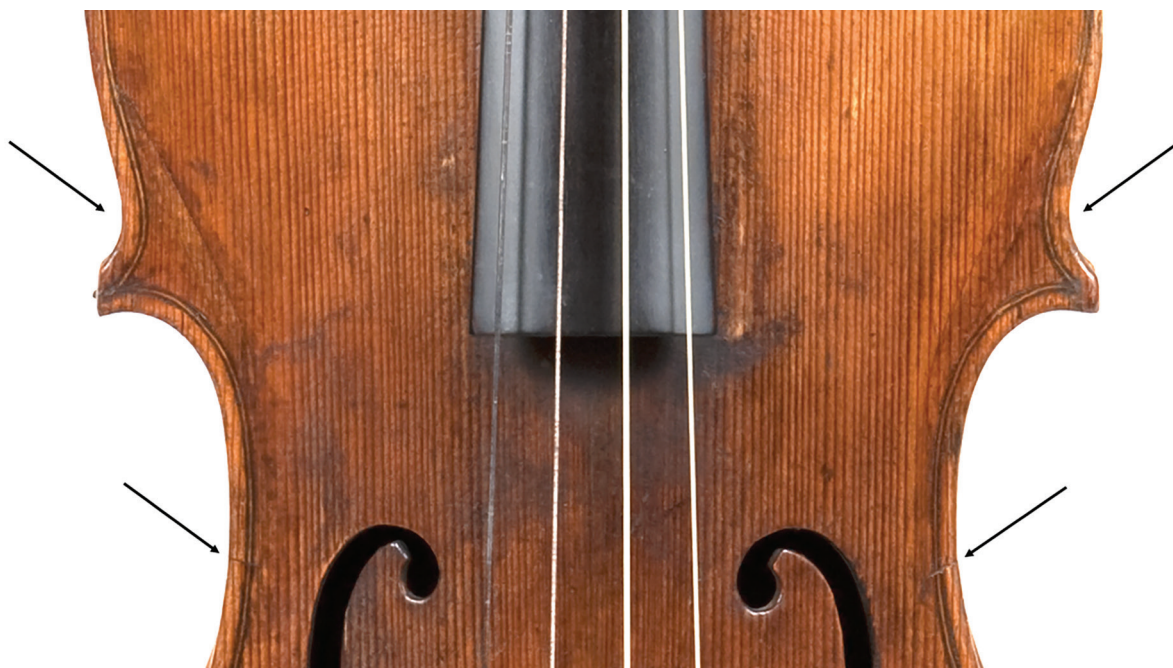
Figure 7. Viola attributed to Hofmans, corner inserts and incision of the C-bouts.
