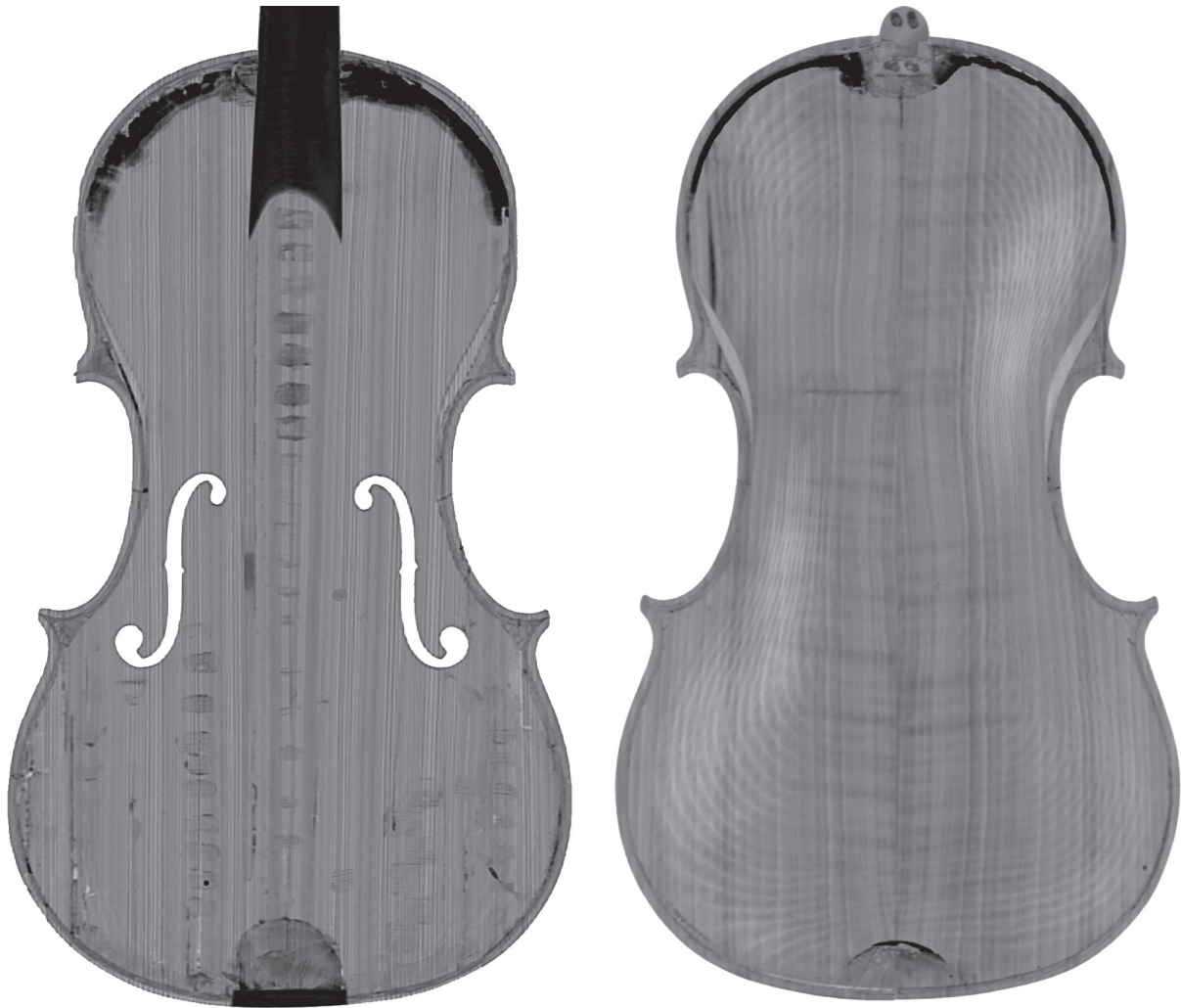
Figure 10. Views of the CT scans: soundboard of the viola attributed to Hofmans at a thickness of 2.1cm and back at a thickness of 2.2cm.
